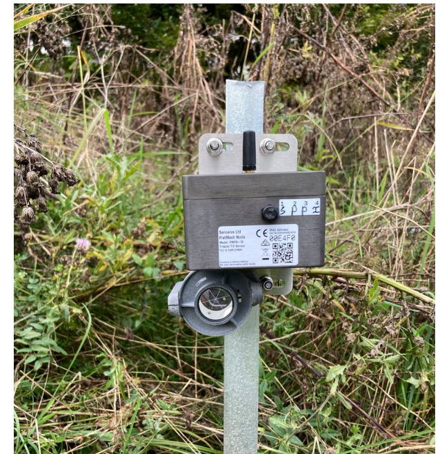
Picture 2: Stake mount with Triaxial Tilt Sensor Node and prism
